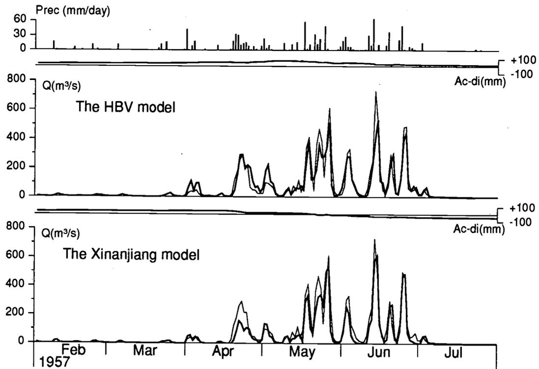
Figure 6. Example of Applications of the HBV and Xinanjiang Models to the Hushile Basin in China and Bird Creek in the U.S.A. Prec = precipitation, Q = computed (thick) and recorded (thin) discharges, Ac-Di = accumulated volume error of runoff.
