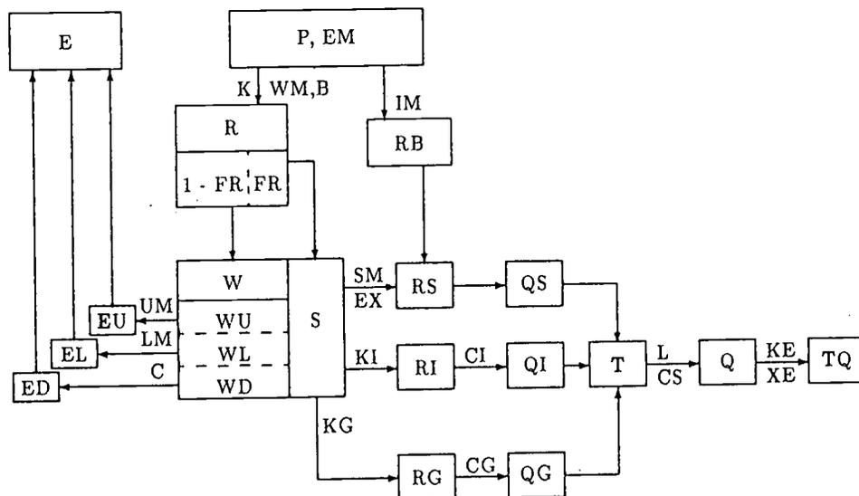
Figure 2. The Flow Chart of the Xinanjiang Model as Applied to One Subbasin (after Zhao, 1992).
