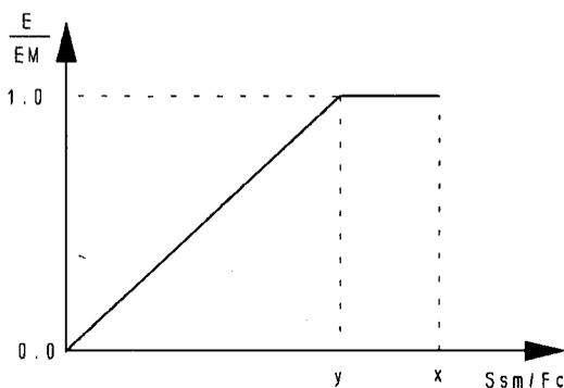
Figure 3. The Evaporation Mechanism of the HBV Model, where  $Ssm$  is the Soil Moisture,  $Fc$  is the Capacity of  $Ssm$ ,  $E$  is the Actual Evaporation, and  $EM$  is the Potential Evaporation Rate.
