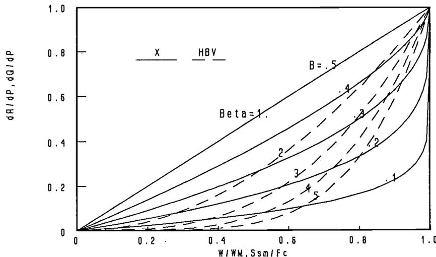
Figure 5. The Relation Between the Runoff Coefficient and Soil Moisture (solid lines represent the Xinjiang model and the dotted lines the HBV model).
