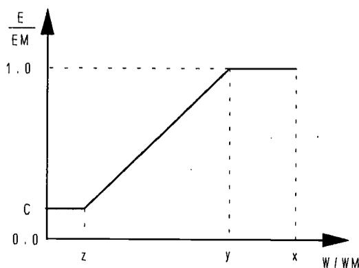
Figure 4. The Evaporation Mechanism of the Xinanjiang Model, where  $W$  is the Total Soil Moisture,  $WM$  is the Capacity of  $W$ ,  $E$  is the Actual Evaporation, and  $EM$  is the Potential Evaporation Rate. The curve is strictly valid for the drying phase only.
